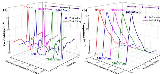
Figure. 4 THz spectra of FC-40 under different electric fields. (a) THz time domain spectra and (b) THz logarithmic frequency domain spectra
