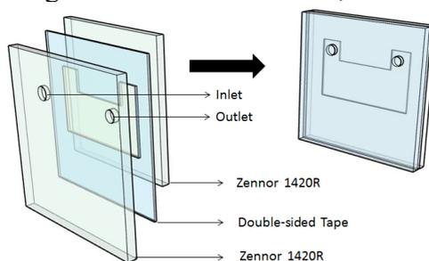
Figure. 1 Schematic diagram of microfluidic chip manufacturing process
