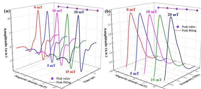
Figure. 6 THz spectra of FC-40 under different magnetic fields. (a) THz time domain spectra and (b) THz logarithmic frequency domain spectra
