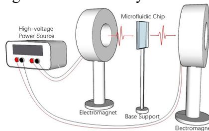
Figure. 3 Schematic diagram of external magnetic field device
